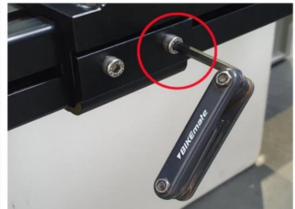
Step 2: Loosen the screw at the bottom.
