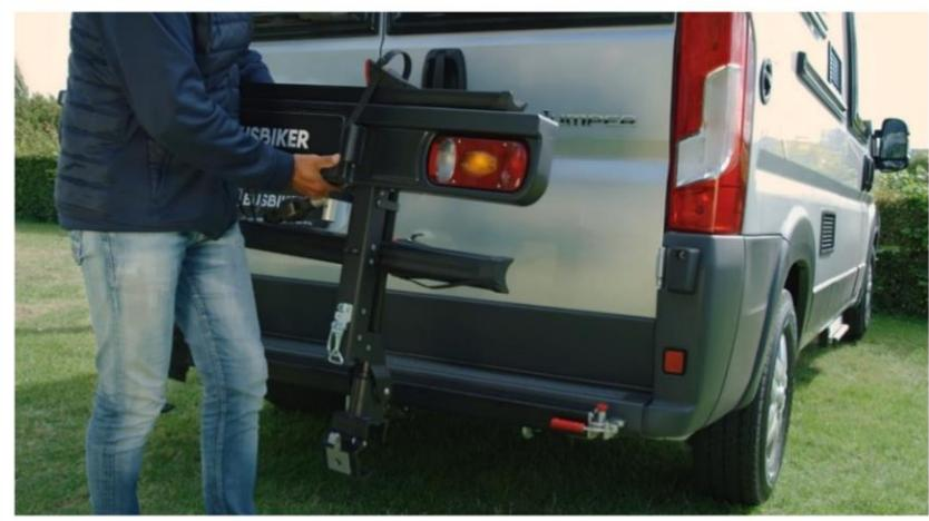
Step 1: Loosen the screws at the back.
